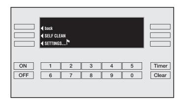
The default oven settings can be changed in the function "SETTINGS". In this function you can customize the oven to suit your preferences. Settings may be adjusted by touching the appropriate touch control.
